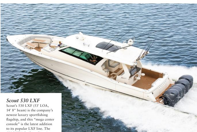
14' 8" beam) is the company's newest luxury sportfishing flagship, and this "mega center console" is the latest addition to its popular LXF line. The 530 LXF is built on Scout's carbon fiber, epoxy-infused, double-stepped, fuel-efficient hull. The epoxy infusion process provides strength for stability while reducing overall weight. Electrically actuated port and starboard beach platforms, when deployed, extend the cockpit width to 17 feet for more room to entertain and play in the water.
