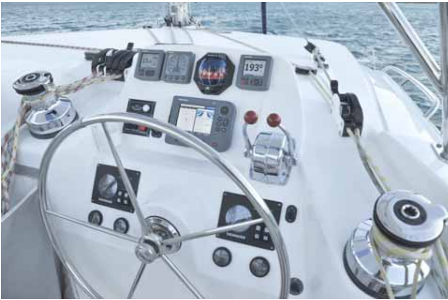
The helm station to starboard has wheel, engine controls, sail controls, and electronics all close at hand.
